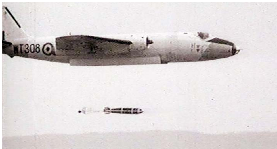
WE177A test round released from a Canberra B6. The parachute drogue has deployed © MoD
