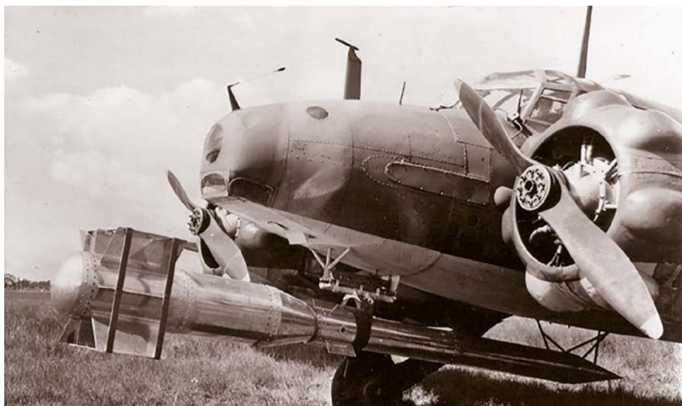
An Anson of NARIU, assisting with trials of the Liquid Oxygen-Petrol, Guided Anti-Aircraft Projectile, (LOPGAAP) which was suspended backwards on the bracket used to hold the ASH radar, for telemetry tests, at RAF Christchurch in May 1945.
