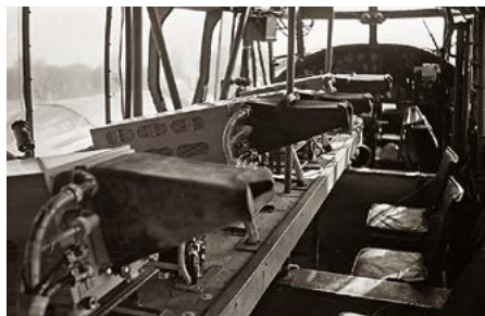
Anson fitted out as an AI Mk IV Radar Trainer for three students and one instructor
