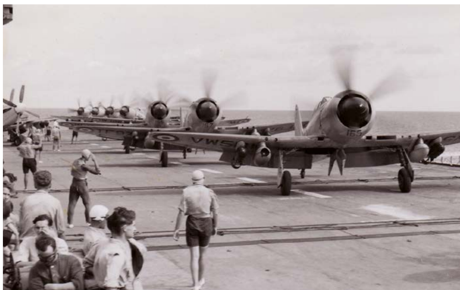
Sea Furies running up for a ground attack mission, note the 500lb bombs on the wing hardpoints.
