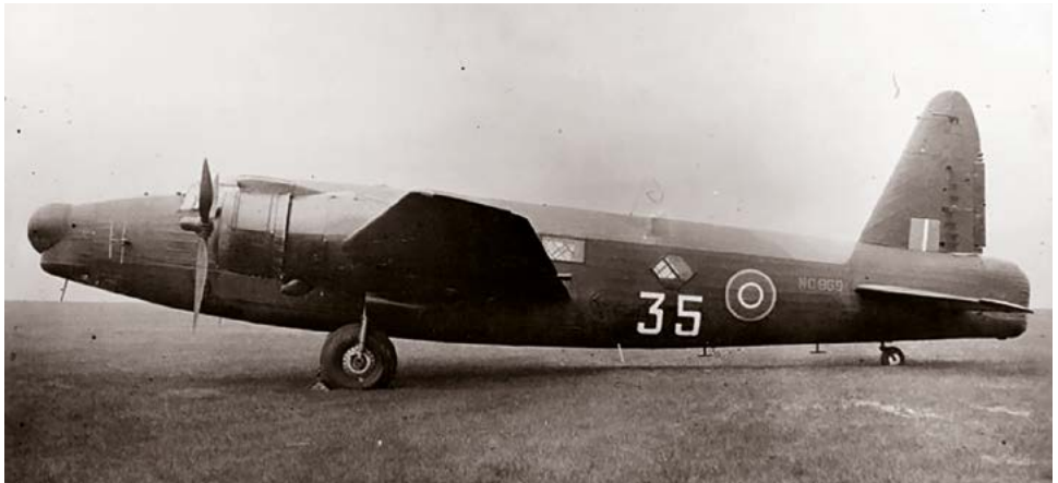
Wellington T Mk XVII flying classrooms for AI training. The NARIU Team was responsible for the installation of the AI Mk X radar set (American built 10 cm SCR720).
