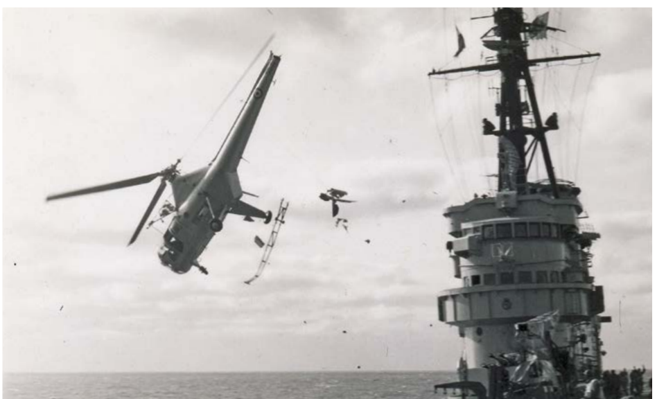
Westland Dragonfly with detached tail rotor crashing into the sea. No comments were on this photo about the fate of the crew or the circumstances of what happened to cause this crash.
