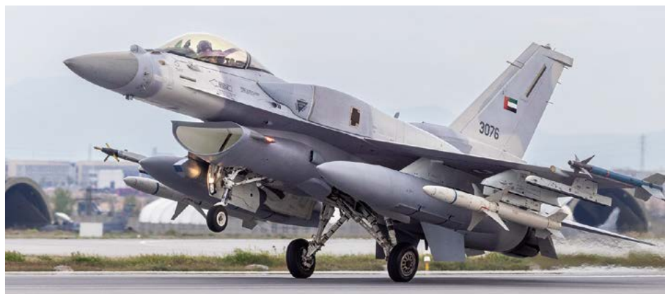
UAE F16, note the AGM-88 high speed anti radiation missiles under each wing. © Tim Smith
