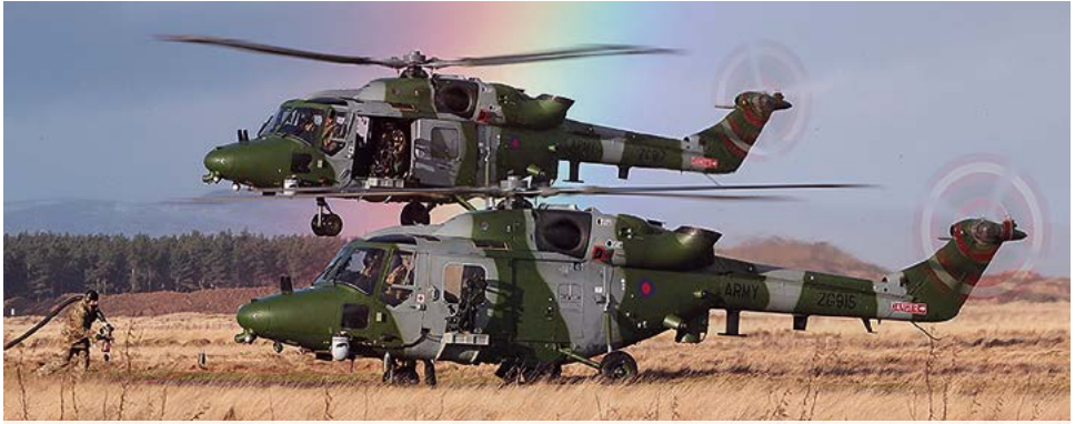
Army Lynx Mk 9As. Note the up-turned exhaust pipes © Andy Walker
