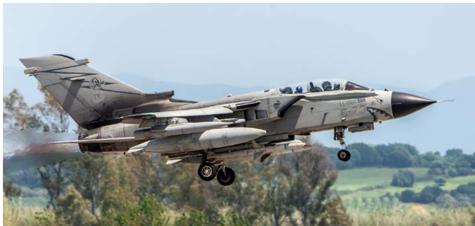
Panavia Tornado IDS of 6 Gruppo, Aeronautica Militare (Italian Air Force) carrying two AGM-88E AARGM missiles on the under fuselage weapon stations. © Richard Macauley
