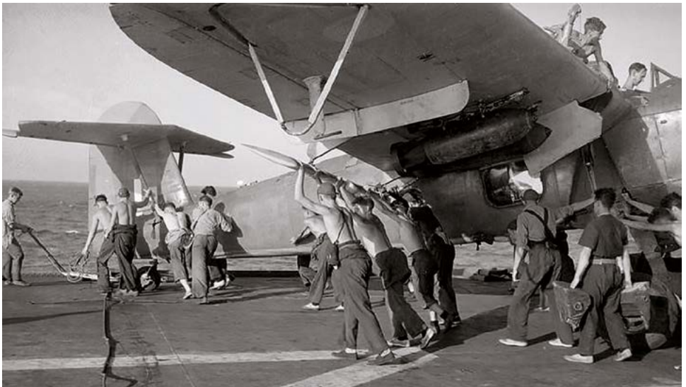
A Barracuda being manhandled on the flight deck of HMS Illustrious Aug 1944. Note the tail wheel steering arm used for manoeuvring. The flaps are set at the 'Dive' position. Also deployed under the wing is the V shaped handle, used to aid the wing fold process. Note also the air speed pitot head mounted on its stanchion on the outboard wing.
