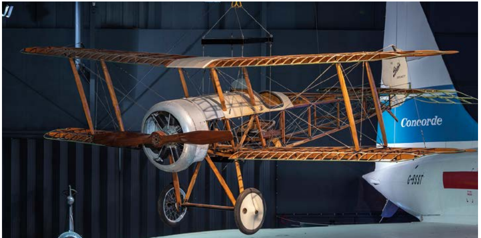
The completed framework of the Bristol Scout now hanging in Hall 4 of the Fleet Air Arm Museum. The background of Concorde G-BSS7 offers a glimpse of a different technology. © Richard Macauley
