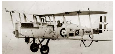
DH9A, modified by Westland, it used the American 400hp (300 Kw) Liberty engine.
