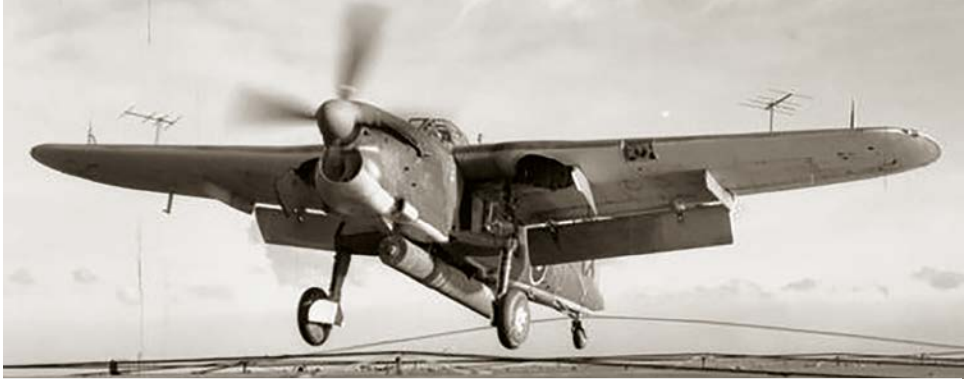
Catching a wire aboard HMS Vengeance with full 'Down' flaps deployed. Note the Radar aerials on the wing upper surfaces. This aircraft appears to be carrying a 1640lb mine.
