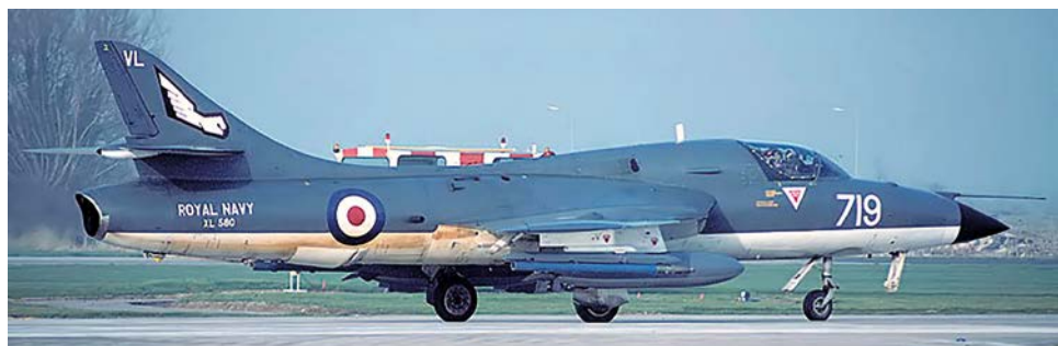
This image of XL580 about to launch from RNAS Yeovilton clearly shows the re-designed nose to accommodate the Blue Fox radar. ©Mick Freer/Mark Russell
