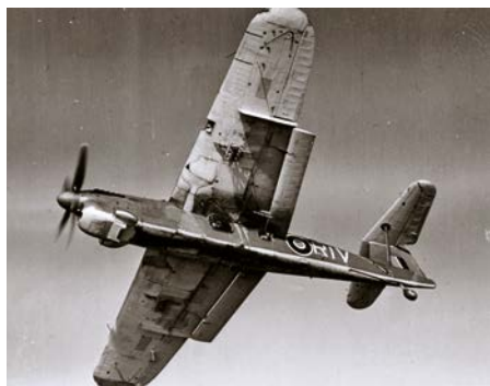
Underside view of Barracuda from 814 Squadron. Note the flaps at the Normal - neutral position.
