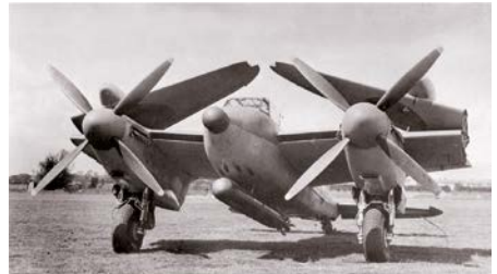
Prototype TR.33 Sea Mosquito 'LR387', with folded wings, torpedo and drop tanks load out and an early 'thimble' style radome. © Dan Shumaker Collection
