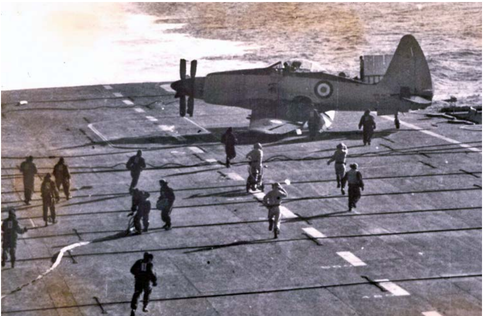
5. A fortunate escape from a potentially fatal landing incident. This final photograph shows the damage to the propeller blades from contact with the deck. © J Perring private collection
