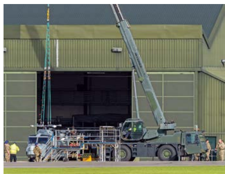
JADTEU and RNAS Yeovilton staff assessing a Wildcat for future transportation as an under-slung load. © Richard Macauley
