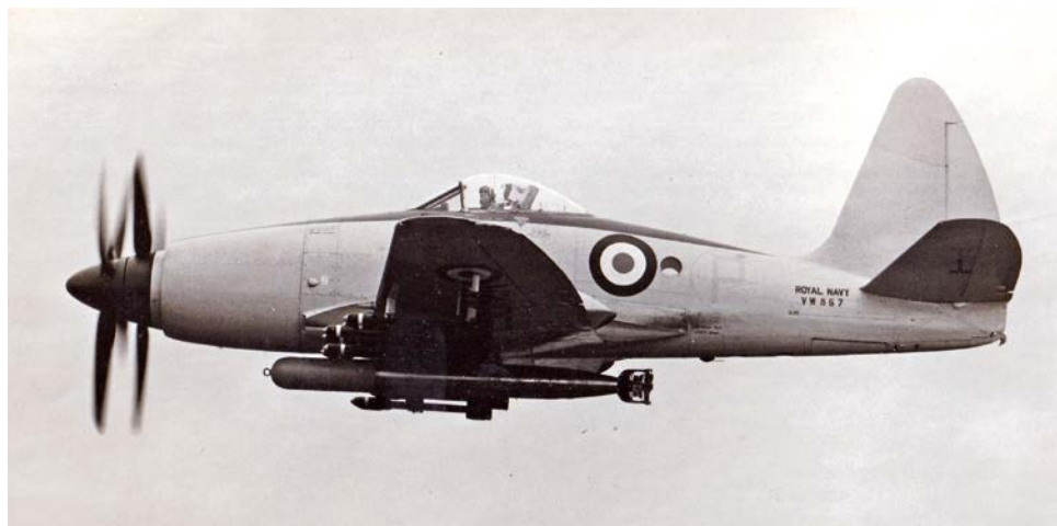
Wyvern VW867 again in flight, showing a potential weapon load. © Westland Aircraft
