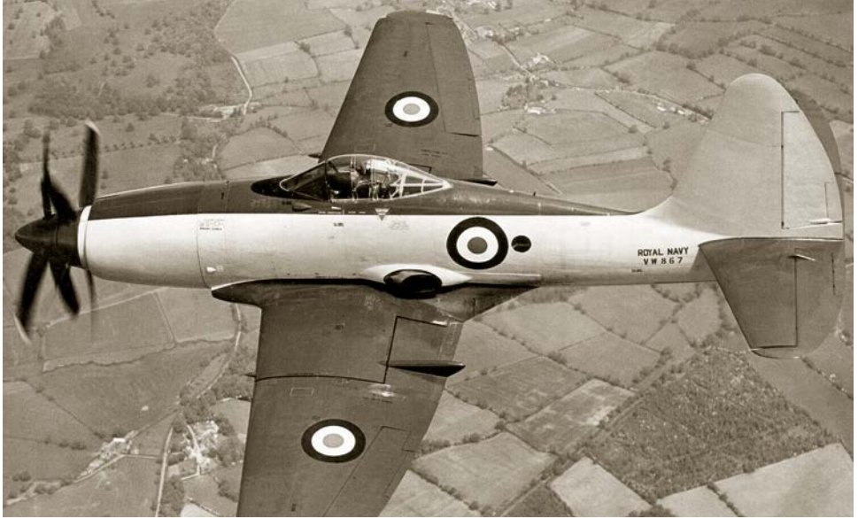
A fine picture of Wyvern VW867 in flight, the first of 20 pre-production aircraft and showing the contra-rotating propellers and the jet pipe of the Python engine. © Peter de Jong Collection
