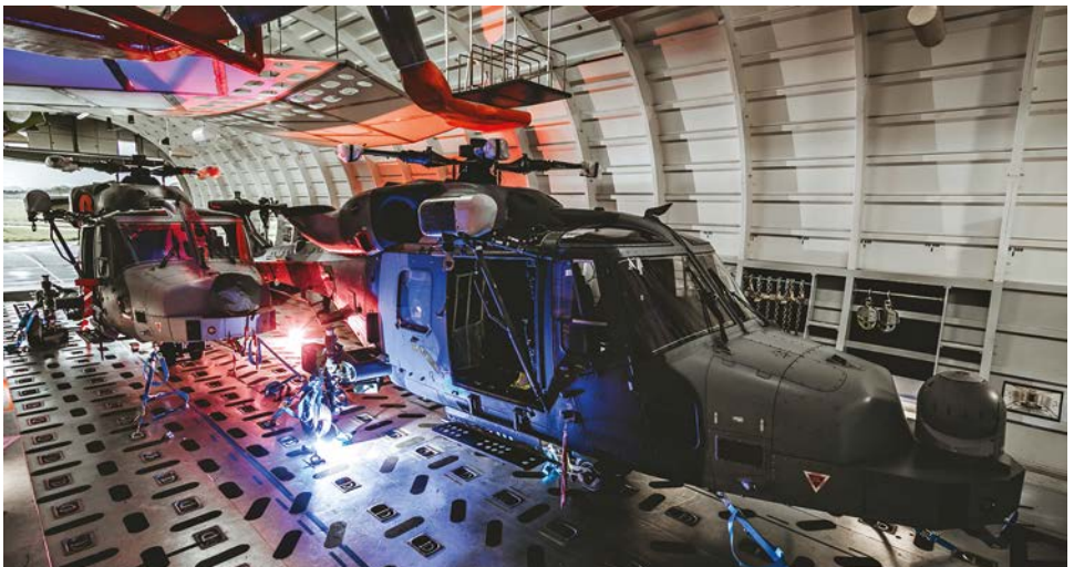
A pair of AAC Wildcat AH1s loaded aboard JADTEU's C-17 cargo hold airframe mock-up at Brize. © JADTEU
