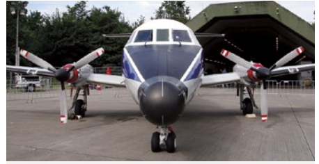
The distinctive shapes of a Jetstream T2 nose and the Turbomeca Astazou engines.
