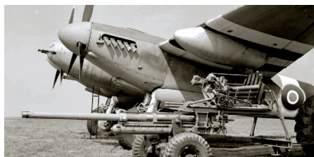
Wheeled Molins 6-pdr gun to demonstrate the size of the weapon against the airframe.
