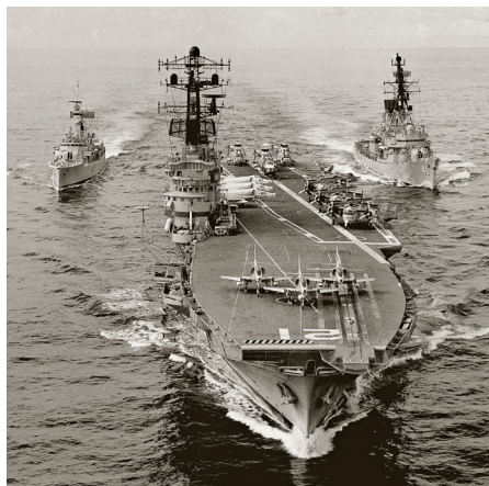
The former Majestic class light fleet carrier HMAS Melbourne was sold to China for scrap. She was studied for development of a future Chinese carrier force.
