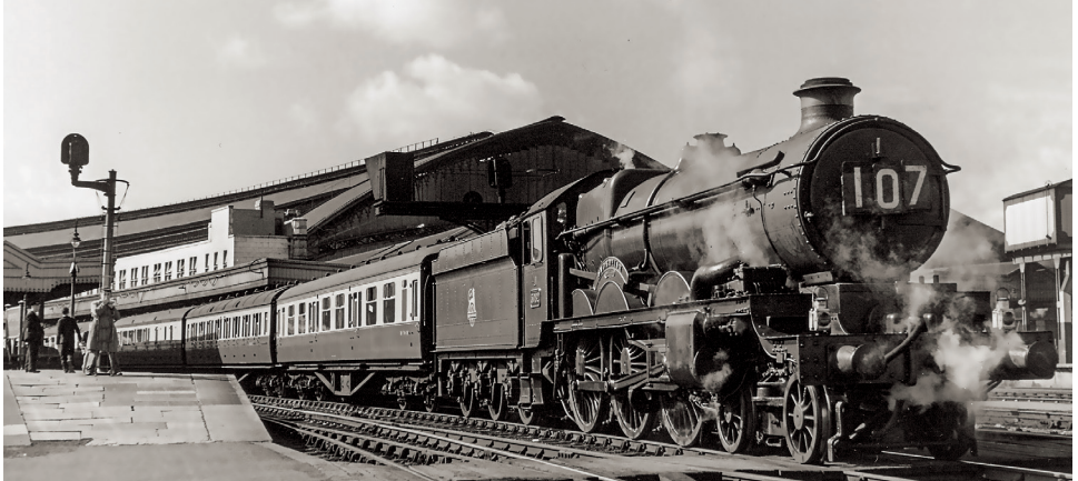
GWR-designed 4-6-0 'Castle' 5082 Swordfish powers away from Bristol Temple Meads on a summer Saturday Kingswear-Paddington express in the early 1950s. © Great Western Trust Didcot/George Heiron
