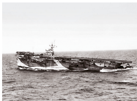
HMS Nabob 'dragging' her stern while returning back to port after being torpedoed.
