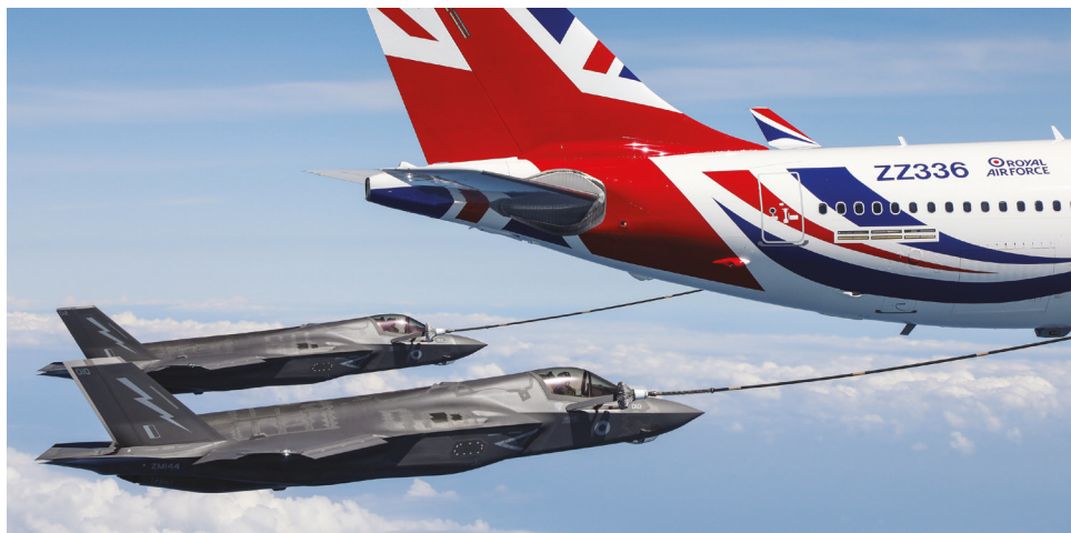
617 Squadron F-35B Lightnings conducting air-to-air refuelling over the North Sea. © Crown Copyright
