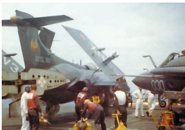
A busy scene as armourers in red surcoats wheel 540lb bombs to the aircraft. © Malcolm Smith
