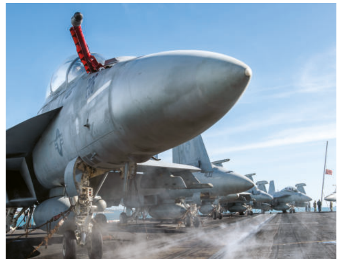
CVN-75 main flight deck and note the steam coming from the catapult rails.
