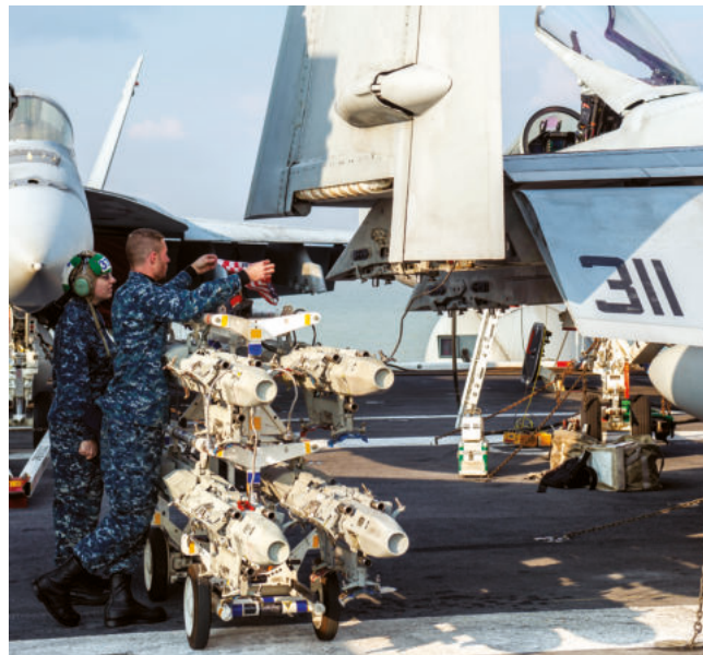
Preparing to fit weapon Multiple Ejector Racks (MER) to F18E aircraft.
