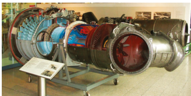
A sectioned example of the Pegasus (now the Rolls Royce Pegasus after industry amalgamation). Components from left to right include the wide diameter LP compressor. A mounting ring indicating the location of the forward nozzles, the HP compressor, the LP shaft, the two turbine stages and the bifurcated jet pipes connecting to the rear nozzles. Ducting and combustion chambers have all been removed. Photograph by Jaypee.
