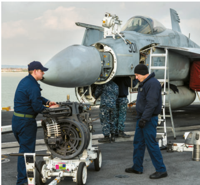
Servicing the 20mm M61 rotary cannon.
