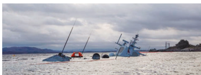
HNoMS Helga Ingstad nearly fully submerged after holding cables snapped and she slipped into deeper water. © Norwegian Coastal Administration
