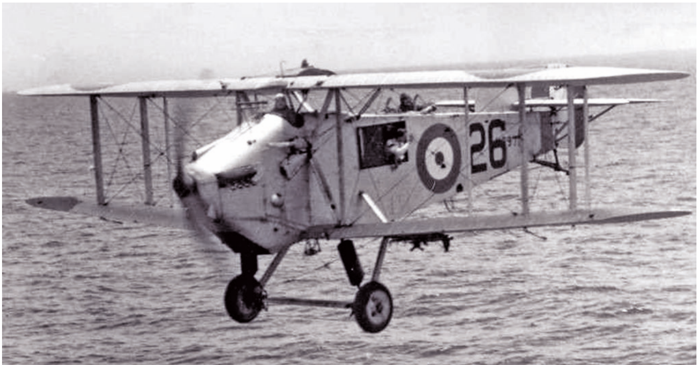
Avro's offering for a carrier-based fleet spotter and reconnaissance aircraft as competition to the Blackburn Blackburn. © asisbiz
