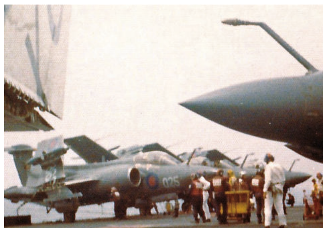
Buccaneer 025 (centre) is armed with two 540lb bombs on a tandem beam under each wing. © Malcolm Smith
