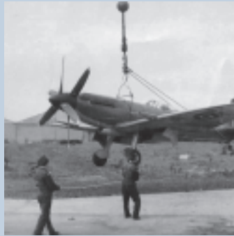
Seafire Mk 47, at an unidentified air station. The RR Griffon engine replaced the Merlin and needed two contra-rotating propellers to absorb the extra power. The mid-1930s designed fuselage was not up to the stresses of deck operations and the type was retired after a final operational period in the Korean War, p37
