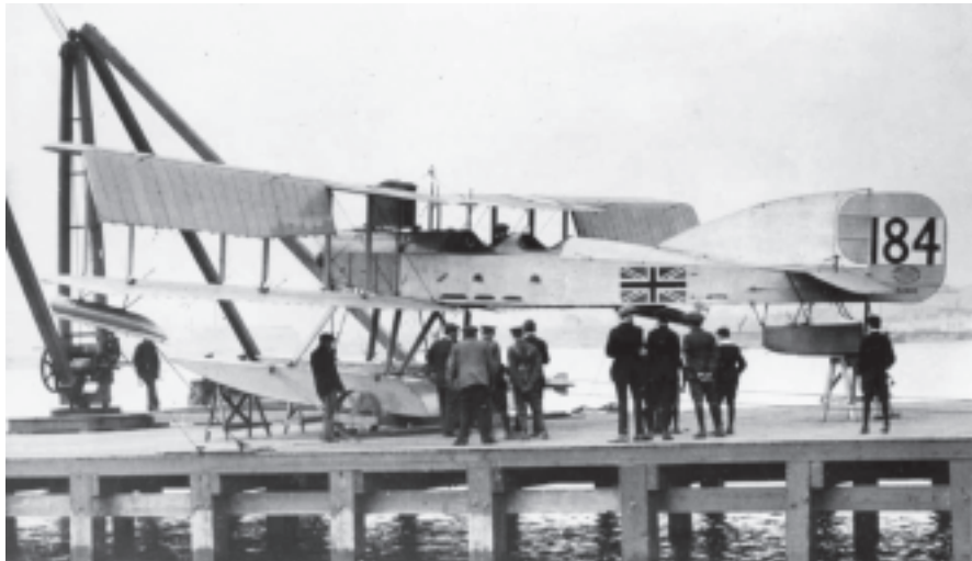
Short 184, 184, at Rochester March 1915. The original construction number S.106 can just be seen on the rudder. Note the unsupported upper wing ailerons. (FAAM JMB/GSL)
