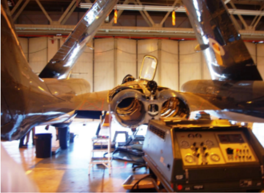
An unusual view of Navy Wings' Sea Vixen, with both engines removed. Photo: Ernest Lear
