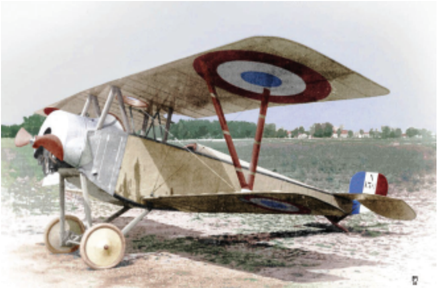
Nieuport 10, two-seat scout and reconnaissance aircraft. Colorised picture, attributed to NiD.29 - Own work
