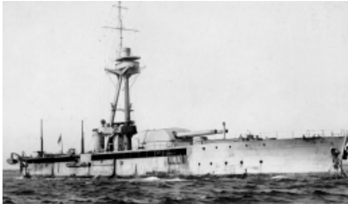
HMS Roberts, a monitor with a twin 14 inch turret, deployed to the Dardanelles in 1915 for shore bombardment of Turkish positions. Dacre spent some time "spotting" for the Roberts' guns and was subsequently detached to the vessel with his aircraft to mount the torpedo attack narrated in this article.
