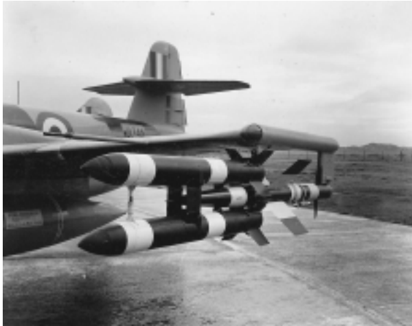
Fairey Fireflash beam-riding missile on the port wing of a trials Meteor. The missile itself was unpowered, being boosted to Mach 2 before the rocket boosters were jettisoned. The missile had a radio receiver in the tail to receive guidance signals from the aircraft.
