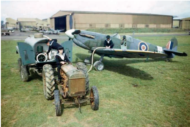
Seafire being refuelled from a towed bowser at Yeovilton in September 1943. Photo Lt E A Zimmerman
